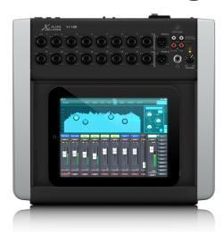
18-Channel, 12-Bus, 6 Aux Digital Mixer for iPad/ Android Tablets with 16 Programmable MIDAS Preamps, Integrated Wifi Module and Multi-Channel USB Audio Interface.
